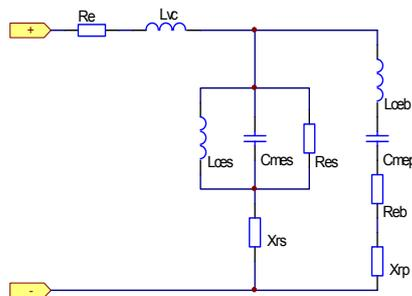
Now there are some other complicating elements that would make for a complete mechanical and acoustical model, such as the mutual coupling of the driver and port, etc., but for the electrical model the above suffices quite well for predicting reality.
