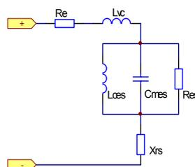
Now, the relative values of these components depends upon the magnitudes of the physical values times a transformation factor. That transformation factor is the electromagnetic transduction factor, proportional to the  $Bl$  product (the product of the length of the wire  $l$  immersed in the magnetic field  $B$ ), measured in  $N/A$  (or  $T/M$ , if you will). So, IF we know the magnitudes of the physical components, we can easily calculate their electrical equivalents:
